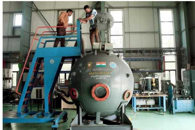
A prototype of the MATSYA 6000, a submersible made by the National Institute of Ocean Technology in Chennai. The final version is expected to undertake a journey to a depth of 6,000 metres. R. RAVINDRAN
